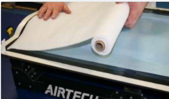
Breather fabric positioned over the release film
