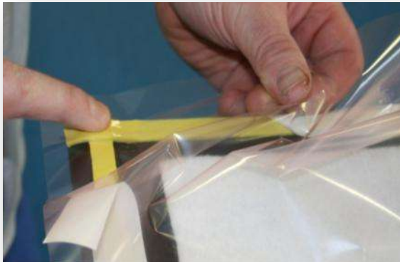
AT200Y being used to form a seal between mould tool and vacuum bag
