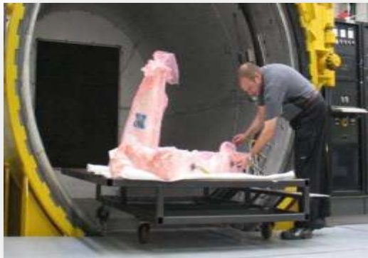
Moulds envelope bagged for Autoclave curing
