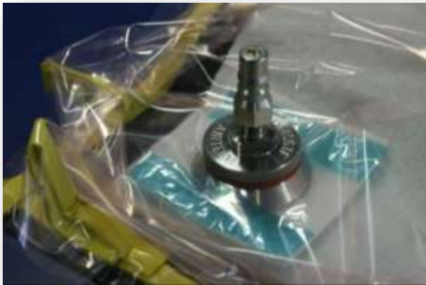
Through bag connector used to connect vacuum hose to vacuum bag
