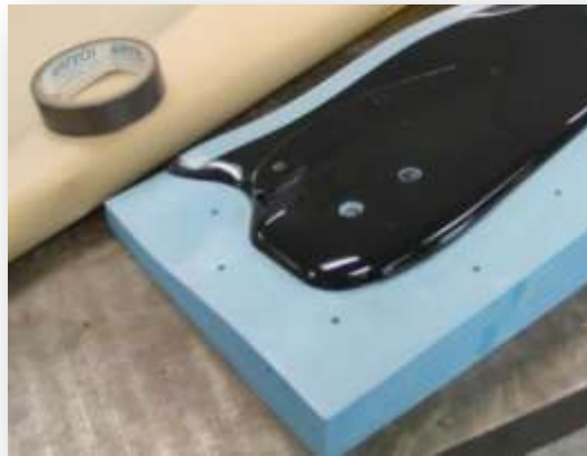
Tooltec CS5 & Teflease provides a smooth release surface on master patterns
